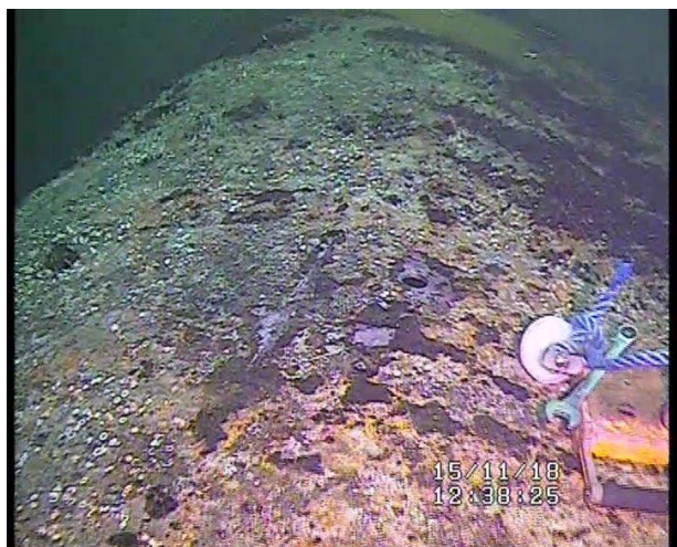
Figure 21. The hull of the shipwreck Sandön, notice the drilled hole in the middle of the photo. Photo: Marine Works AB/Secure Rescue & Safety AB.
