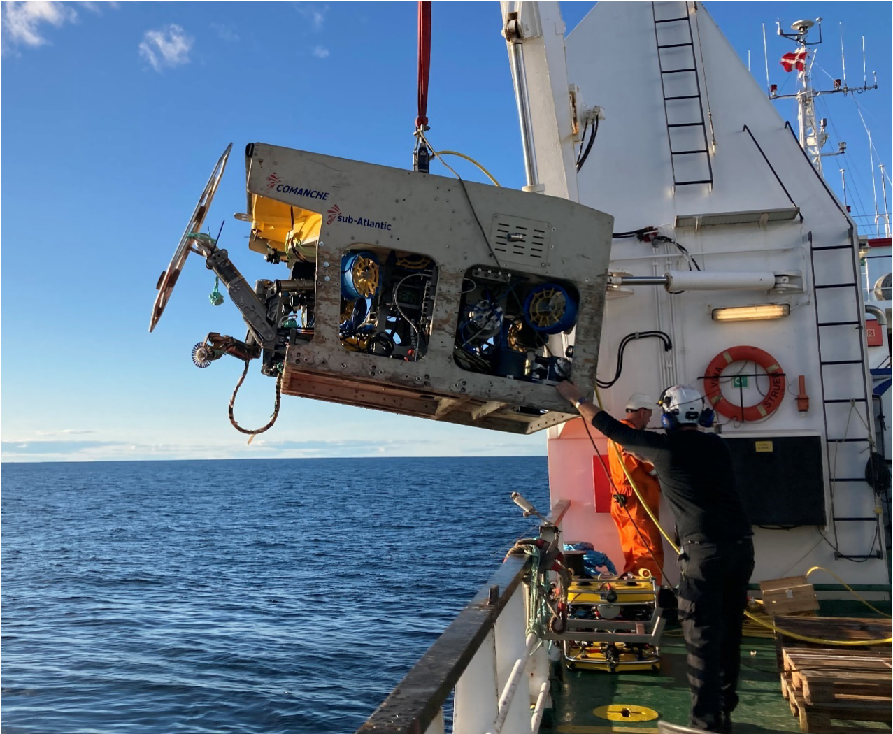
Figure 50. Large ROV onboard work vessel Vina used for survey and oil removal operation of the wreck Rone in 2022. The ROV is equipped with two manipulator arms, one for cleaning the hull of the wreck from organic debris and old paint, and one for carrying drilling equipment (not attached in the photo) (Photo: JF Lindgren).
