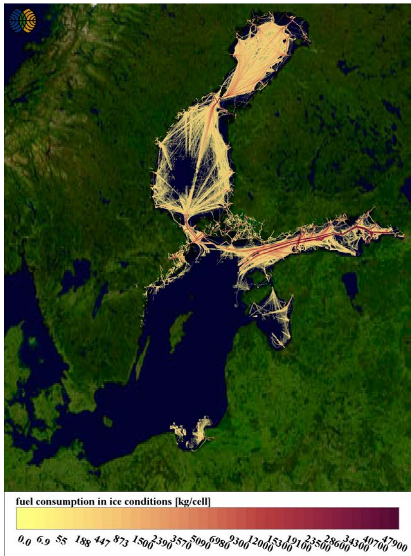
Figure 12 Total annual fuel consumption (kg) in ice conditions in the Baltic Sea in 2023
