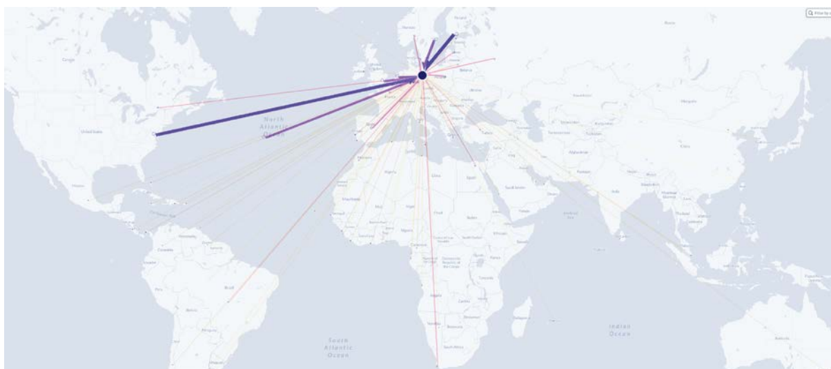
Figure 8 Example of CO 2 emissions of import traffic network of Germany. The width of the arrows and the size of the circles are relative to CO 2 emissions from ships travelling between different countries. For Germany, the largest import emissions were associated with ships coming from Finland, USA, the Netherlands and Sweden.
