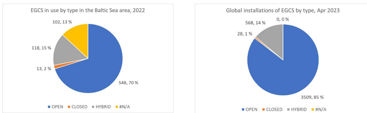
Figure 3 Equipment type of EGCS of the Baltic Sea in 2022(left) and the global (right) shipping fleet in April 2023.
