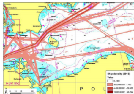
Figure 13: Step 2: AIS data needs to be analysed to designate ship corridors.
