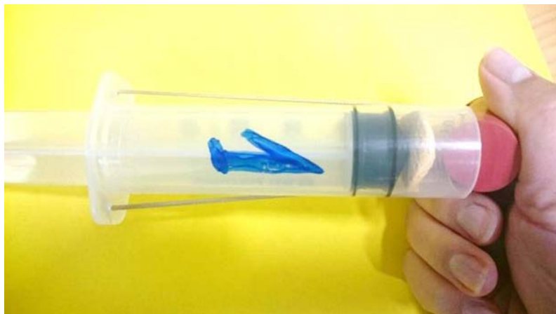
Figure 1: Modified syringe sampling device (photo: A. Zaiko)
