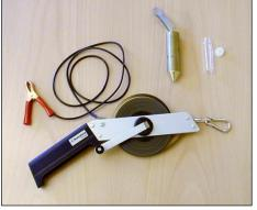
Sample collector with steel measuring tape.
