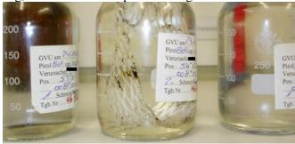
As can be seen in the right-hand picture above, enough oil for the following trace analysis is sampled in this way (right-hand picture, sample on the left: sample taken without Teflon® net, no visible oil; sample on the right: "clean water" taken beside the oil film).
