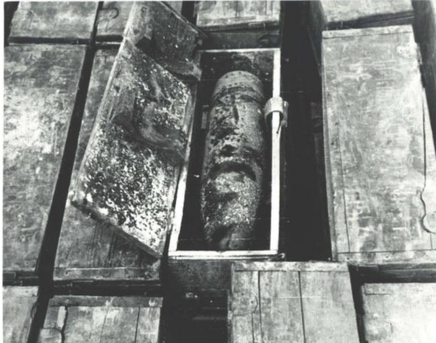
Figure 19: Leaking chemical munitions were sometimes encountered during the trafficking of chemical warfare materials for sea-dumping. This item, leaking sulfur mustard, was encountered during handling in Bremerhaven under control of the U.S. Military Administration in Germany. It was reported to have been decontaminated later. Another general option to cope with such dangerous items was emergency sea-dumping (see text) (HELCOM 2011c).
