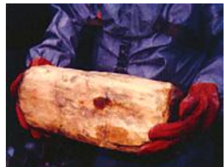
Figure 10: A lump of solidified sulfur mustard from a Spray Can 37 mine, evident by the conserved shape (Picture source: Maritime Surveillance Centre South on Bornholm).
