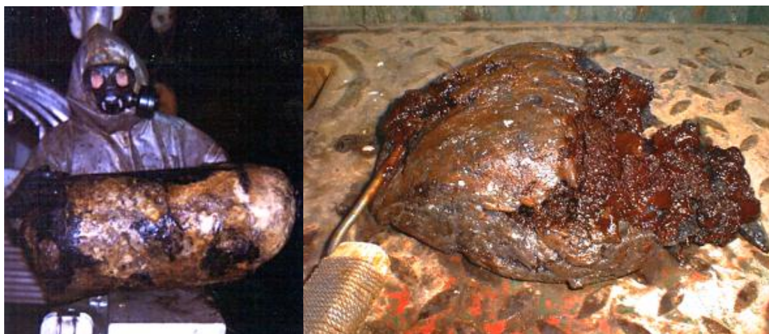
Figure 49: Lumps of solidified sulfur mustard trawled up by fishermen in the waters around Bornholm (left). The 70 kg lump retained the original shape of the KC250 bomb and supposedly contained the bursting charge with 15 kg of explosives inside. The 3 kg lump was found by R/V 'Dana' in 2001 and it could not be ruled out
