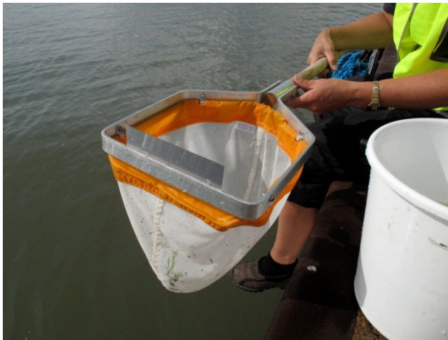
Figure 2. Scraping tool for sampling fouling organisms
