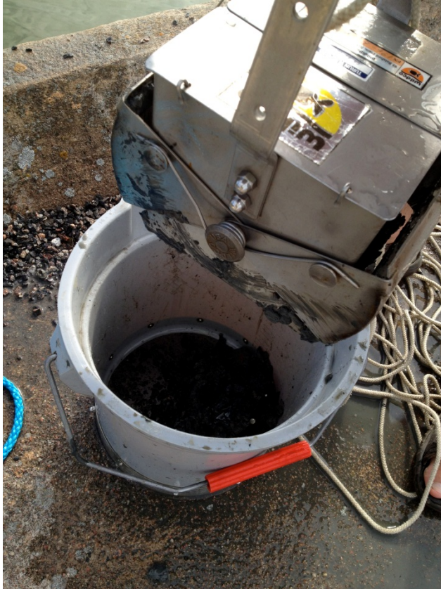
Figure 4 Benthic sample obtained using an Ekman Grab.
