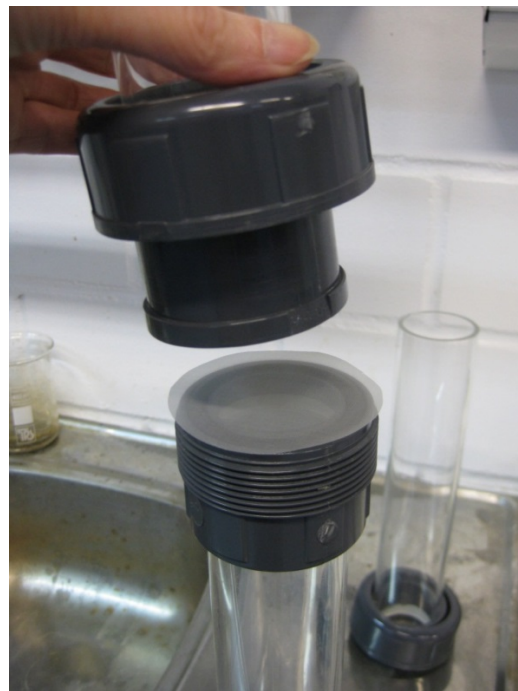
Figure 3. Filter is placed between the screw-on connectors
