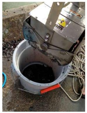
Figure 4. Benthic sample obtained by using an Ekman Grab.
