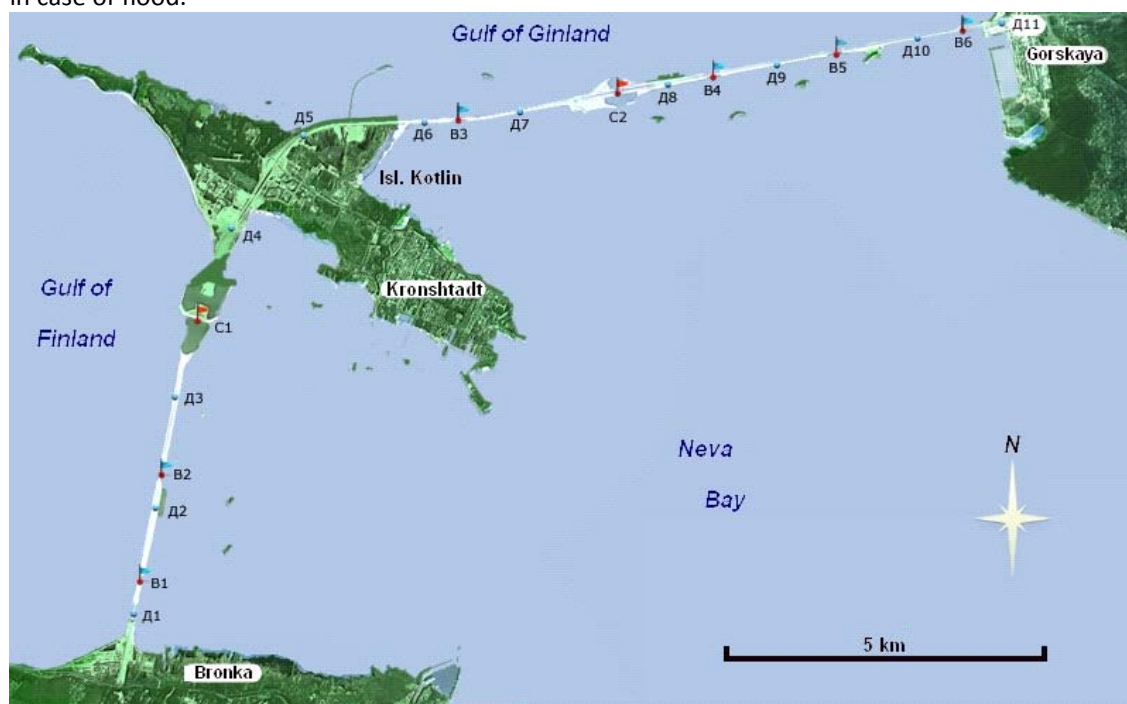
Fig. 4.22.9. Complex of Flood-Defensive Constructions of St.-Petersburg. B1-B6 – water admission gates; C1 and C2 – navigation gates (after Directorate of CDC http://dambaspb.ru ).
