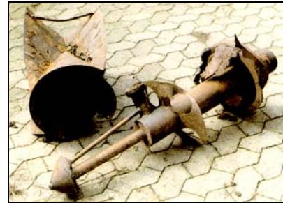
Figure 6 - 63 Central explosive core and tailcone dismounted from such a KC 250 bomb
