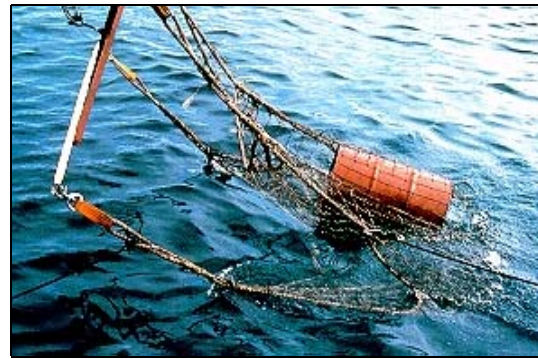
Figure 6 - 34 Collection bag nets for salvage of packaged dangerous goods on the water surface.
