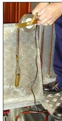
If the oil sample is very small a Teflon® pad can be used. The pad is dipped into the sample and then absorbs a sufficient amount of oil. The whole pad is sent for analysis. The pad is made of Teflon® because other materials might contaminate the sample and disturb the succeeding analysis.
