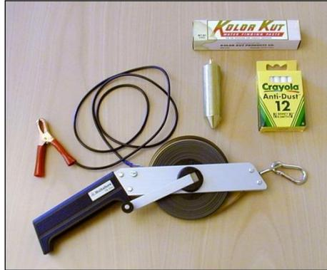
5.21 What is called “**water-finding paste**” may well be used on a normal steel measuring tape to sound the oil-water interface level. The tape is coated with this paste which turns red upon contact with water. The interface level can then be read on the tape. Alternatively the steel tape can be chalked with ordinary blackboard chalk. On some occasions the contrast between oil and water on the steel tape will be better with chalk than with water-finding paste.
