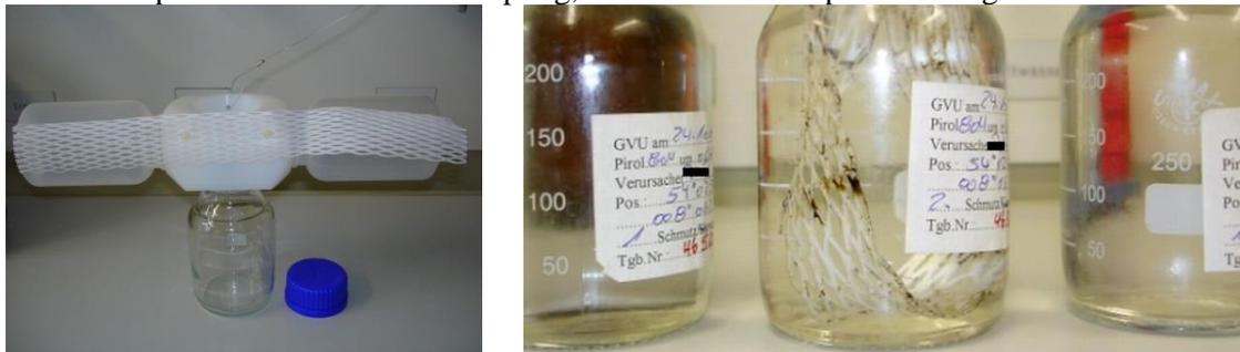
As can be seen in the right-hand picture above, enough oil for the following trace analysis is sampled in this way (right-hand picture, sample on the left: sample taken without Teflon® net, no visible oil ; sample on the right: “clean water” taken beside the oil film).
