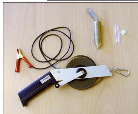
Sample collector with steel measuring tape.
