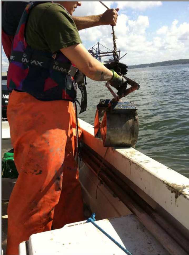
Figure 9 - Handheld Ponar used for benthos sampling.
