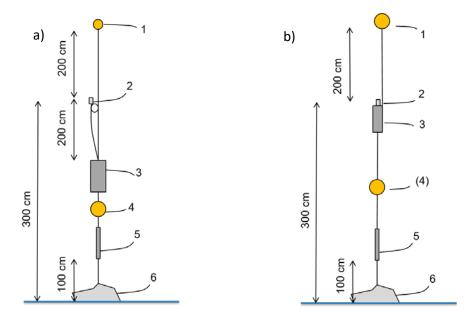
Figure 1. Sketch of two alternative rig design where a) illustrates a rig with a detachable hydrophone and b) a rig with a non-detachable hydrophone that is non-buoyant. 1 hydrophone floatation, 2 hydrophone, 3 hydrophone loggers, 4 floatation element, 5 releaser and 6 ballast weight.
