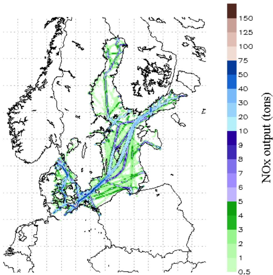
**Figure 1.** NO<sub>x</sub> emission from ships during March 2006.
