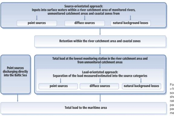
For large rivers (runoff >100 m<sup>3</sup>/s), figures for source apportionment should be given separately for the monitored part and the unmonitored part of the river catchment area.
