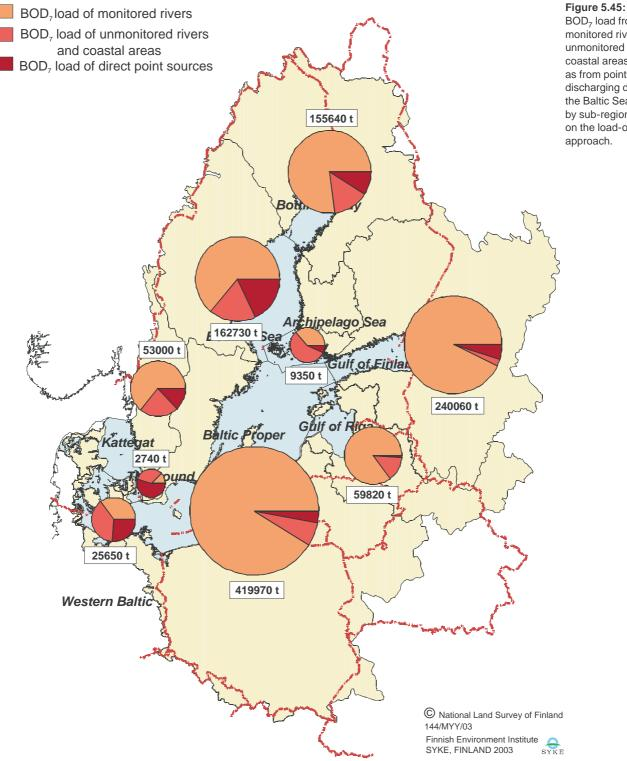
BOD<sub>7</sub> load from monitored rivers. unmonitored rivers and coastal areas as well as from point sources discharging directly into the Baltic Sea in 2000 by sub-region based on the load-orientated approach.
