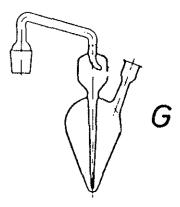
Schematic diagram of the apparatus for wet digestion under reflux with acids
